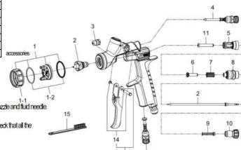
Marked parts are wearable parts.
